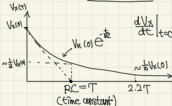
$$\left. \frac{dV_x}{dt} \right|_{t=0} = -\frac{V_x(0)}{RC} \rightarrow \text{tangent line at } t=0$$
