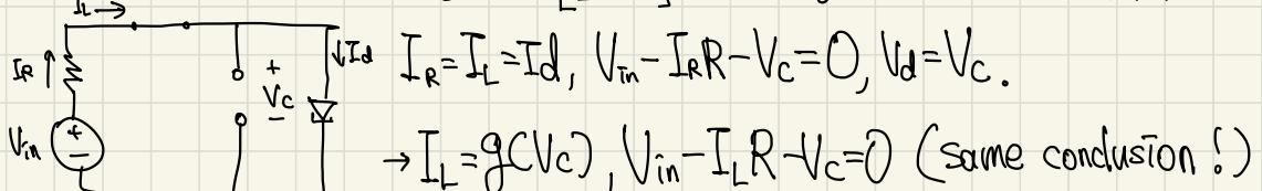
Linearization model:  $J_{\vec{x}}\vec{f} = \begin{bmatrix} \frac{\partial f_1}{\partial x_1} & \frac{\partial f_1}{\partial x_2} \\ \frac{\partial f_2}{\partial x_1} & \frac{\partial f_2}{\partial x_2} \end{bmatrix}$ ,  $J_u\vec{f} = \begin{bmatrix} \frac{\partial f_1}{\partial u} \\ \frac{\partial f_2}{\partial u} \end{bmatrix}$ .  $\vec{f}(\vec{x}(t), u(t)) = \begin{bmatrix} \frac{1}{C}(x_2 - g(x_1)) \\ \frac{1}{L}(u - Rx_2 - x_1) \end{bmatrix}$ .
