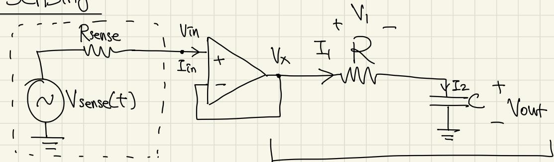
$$V_{\text{in}} = V_{\text{sense}} \quad (\because I_{\text{in}} = 0) \quad \text{Want this circuit to separate}$$
