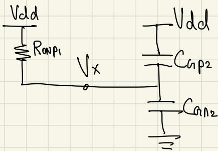
$$V_{x(0)} = V_{dd}$$
