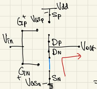
2)  $V_{in} = V_{dd}$ , logic 1 or True
