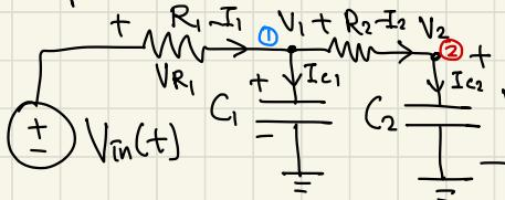
$$KCL: I_2 = I_{C_2}, I_1 = I_{C_1} + I_2$$
