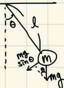
$$\text{Let } \vec{X}(t) = \begin{bmatrix} \theta(t) \\ \omega(t) \end{bmatrix} \text{ where } \omega(t) = \frac{d\theta}{dt}. \rightarrow \frac{d\vec{X}(t)}{dt} = \begin{bmatrix} \frac{d\theta}{dt} \\ \frac{d\omega}{dt} \end{bmatrix} = \begin{bmatrix} \omega(t) \\ \frac{d\omega}{dt} \end{bmatrix} = \vec{f}(\vec{X}(t))$$
