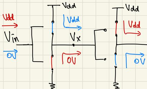
$$1) V_{in} = 0 \rightarrow V_x = V_{dd} \rightarrow V_{out} = 0$$
