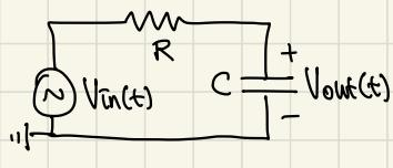
$$\begin{aligned} \textcircled{1} \text{ write sources as exponentials (into phasor domain)} \\ V_{in}(t) &= \frac{V_m}{2} e^{j\omega t} + \frac{V_m}{2} e^{-j\omega t} \end{aligned}$$
