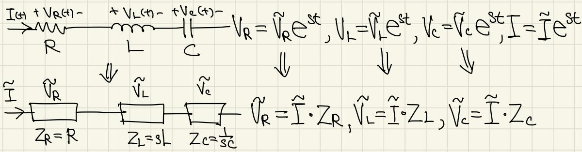
For sinusoids,  $u(t) = U \cos(\omega t + \phi) = U \frac{e^{j(\omega t + \phi)} + e^{-j(\omega t + \phi)}}{2}$
