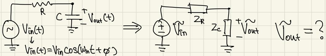
$$\frac{\tilde{V}_{out}}{\tilde{V}_{in}} = \frac{Z_c}{Z_R + Z_c} = H_{LP}(j\omega) \rightarrow \text{transfer function}$$
