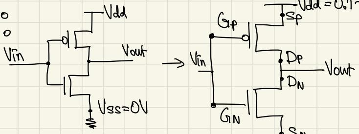
(16B Assumption:  $V_{thn} + |V_{thpl}| \geq V_{dd}$ ,  $V_{dd} \geq |V_{thn}| \geq 0$ )
